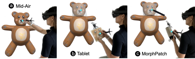
Figure 6: (a) Mid-Air interaction, where the user directly interacts with the virtual object using a pen. (b) Tablet interaction, where the user uses the tablet to control a cursor on the object surface, and the surface is reflected on the tablet. (c) MorphPatch interaction, where the user uses VRScroll and the pen on VRScroll is redirected to the virtual object for manipulation. The transparent layer on the bear’s head represents the surface approximation. Blue cursors represent the pen contact point.
